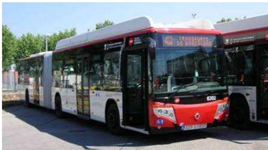
**Irisbus Iveco CITYCLASS CNG 18 m**
